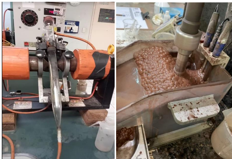
Figure 6 - Typical lab magnetic separation (left) and flotation (right)
