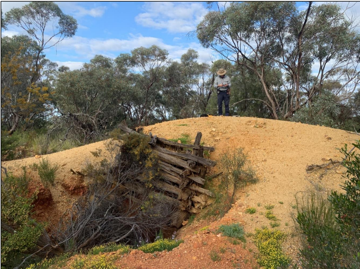
Figure 3: Photograph of AGC geologists standing on mullock heap above the main decline adit which was so deep that the base could not be estimated.
