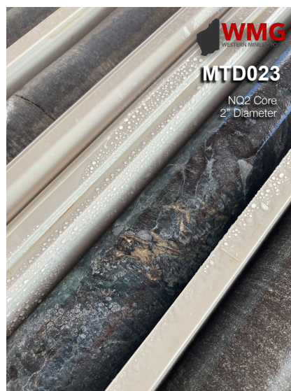
Figure 2: Photos showing examples of visible disseminated sulphides and remobilised sulphide veinlets Note: core is NQ2 being 2 inches or 50mm diameter
