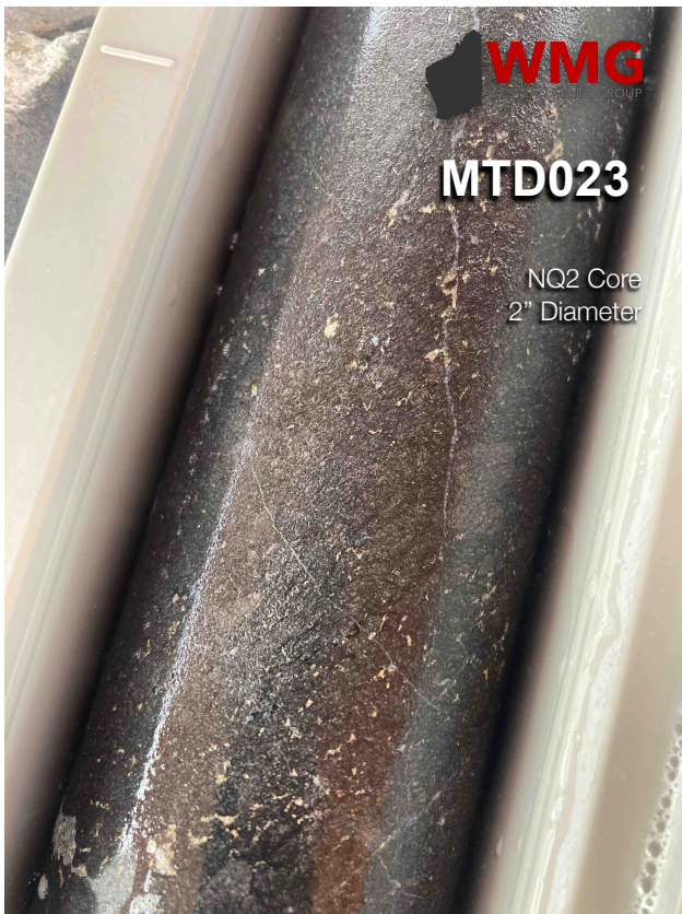
Figure 1: Photos showing examples of visible disseminated sulphides in hole MTD023 with disseminated sulphide forming interstitial blebs between former olivine grains Note: core is NQ2 being 2 inches or 50mm diameter
