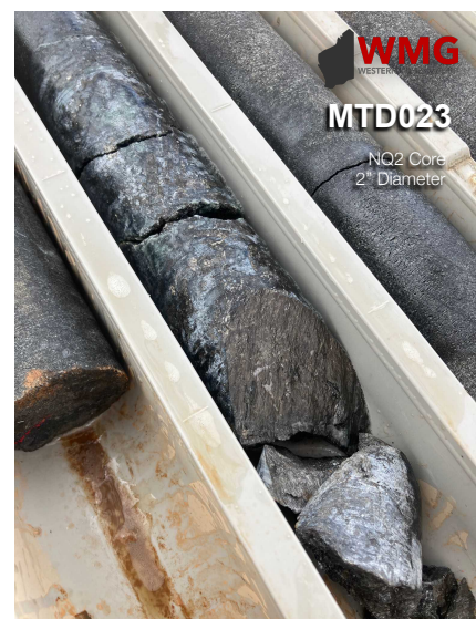
Figure 2: Photos showing examples of visible disseminated sulphides and remobilised sulphide veinlets Note: core is NQ2 being 2 inches or 50mm diameter
