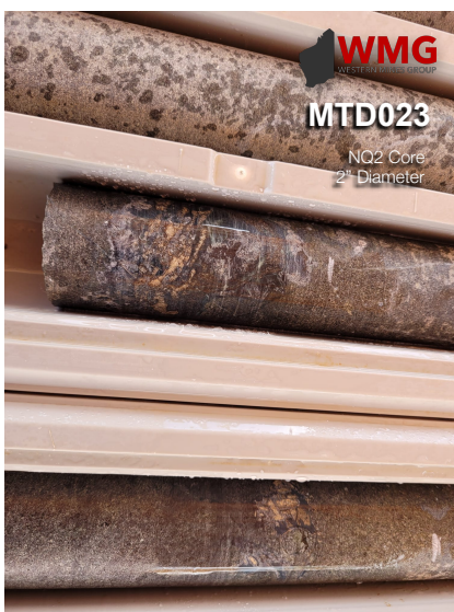
Figure 2: Photos showing examples of visible disseminated sulphides and remobilised sulphide veinlets Note: core is NQ2 being 2 inches or 50mm diameter
