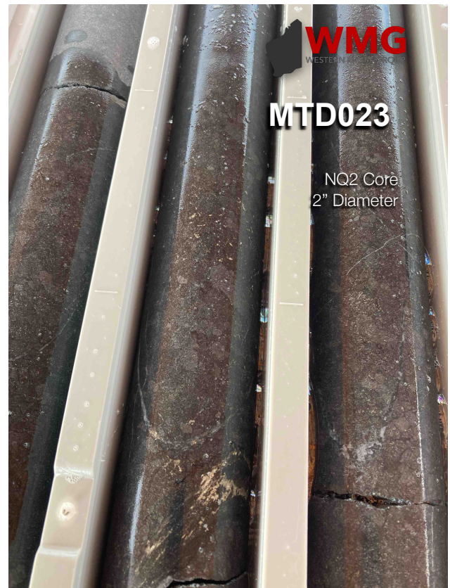
Figure 1: Photos showing examples of visible disseminated sulphides in hole MTD023 with disseminated sulphide forming interstitial blebs between former olivine grains Note: core is NQ2 being 2 inches or 50mm diameter
