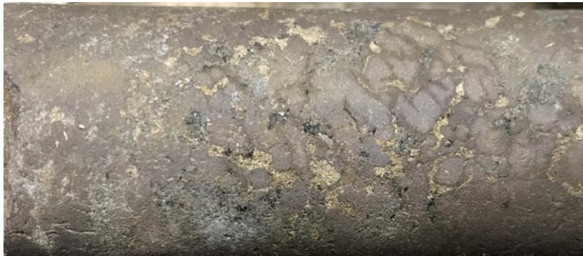
Coarse-grained massive sulphide with pentlandite loops, BH-265-125, from 180m, Brevann Mine. From a 1m sample interval which assayed 3 % Ni
