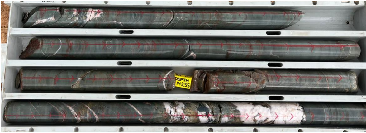
Figure 6. Drill core from 23HEDD003 showing brittle fractures from selective trays showing Quartz-Carbonate-Chlorite veining in the D'Kar Formation above the targeted horizon from 86m to 196m. (1m length boxes)
