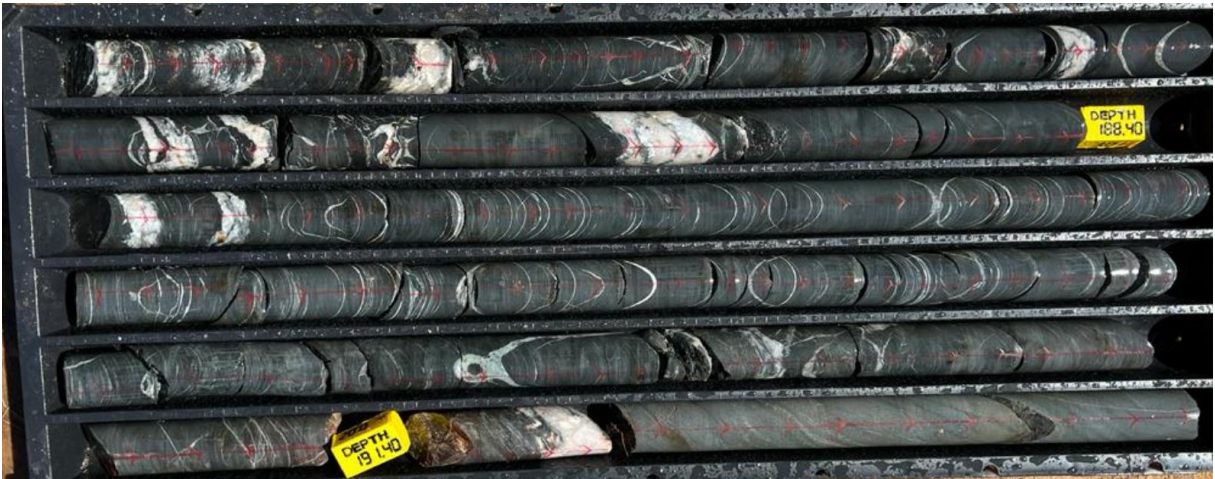
Figure 6. Drill core from 23HEDD003 showing brittle fractures from selective trays showing Quartz-Carbonate-Chlorite veining in the D'Kar Formation above the targeted horizon from 86m to 196m. (1m length boxes)
