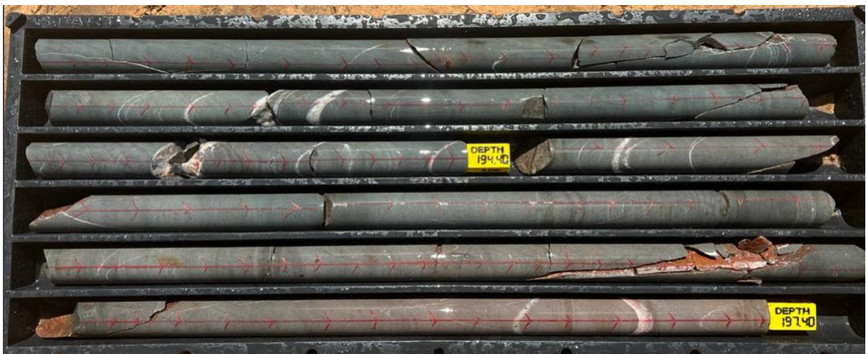
Figure 7. Drill core from 23HEDD003 showing brittle fractures and shearing at the contact at 196.5m of the D'Kar Formation and the Ngwako Pan Formation with minor visible Copper staining.
