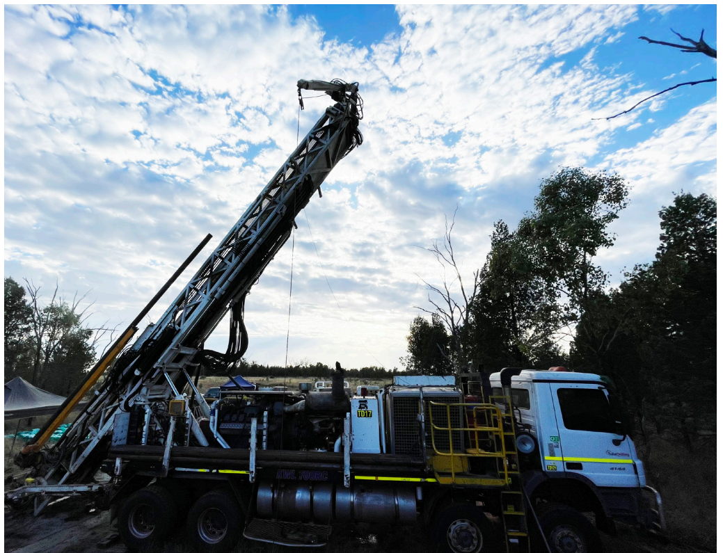
Image: RC Drilling Rig at Tottenham, NSW.
