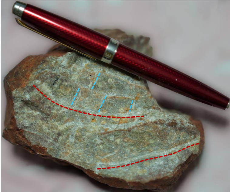
Figure 3: Rock chip sample from location MERI_02. Early vein sets (e.g. blue dash) and altered brecciated groundmass are enriched in molybdenum. Later vein sets (e.g. red dash) are enriched in molybdenum and silver.
