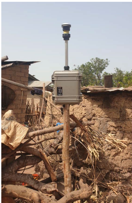
Figure 3. Dust monitoring station on the Simandou North Iron Project.
