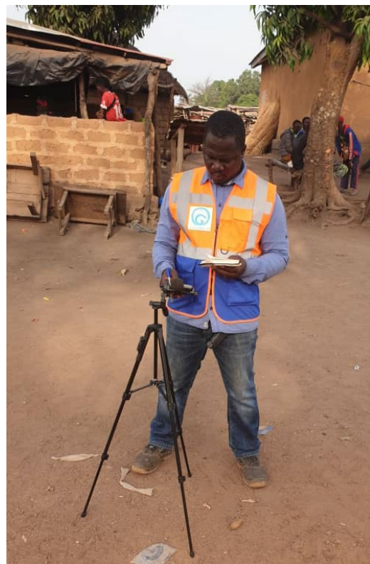
Figure 4. Noise levels being monitored on the Simandou North Iron Project.
