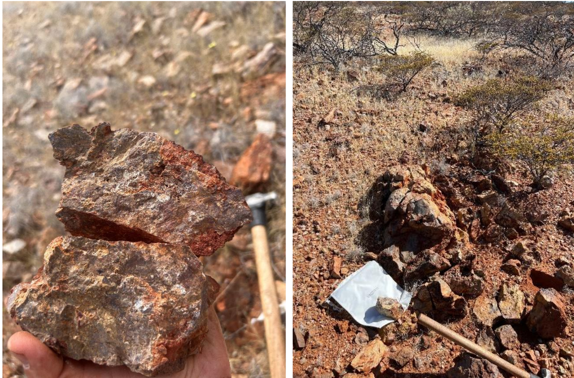
Figure 11: High grade monazite-rich samples MWGS1114 (left) and monazite rich sample MWGS0800 (right) which assayed 15.79% TREO with 2.41% Nd_2O_3 + Pr_6O_{11} and 16.00% TREO with 2.62% Nd_2O_3 + Pr_6O_{11} .
