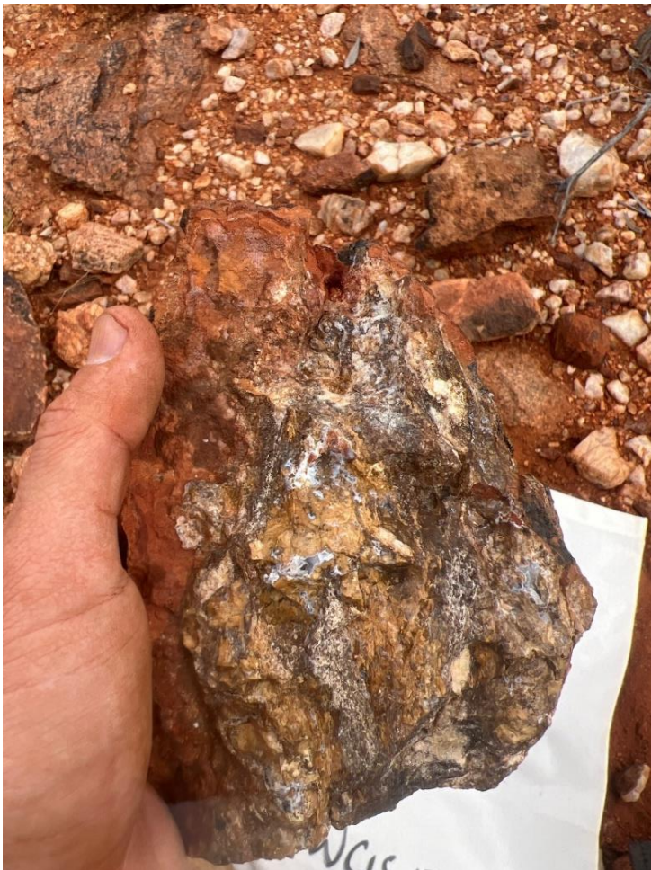
Figure 13: Monazite-rich rock chip sample MWGS1224 which assayed 17.64% TREO with 3.82% Nd 2 O 3 + Pr 6 O 11 .
