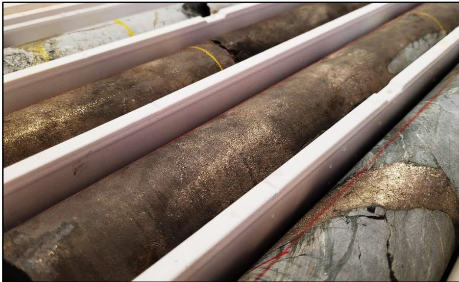
Figure 8: Field photo of massive sulphide in drill core samples from drillhole GSPDD0005, at the GSP Prospect.
