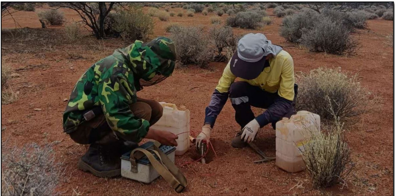
Figure 1: Part of the crew from Echo Vista Geophysical consultants preparing the ground for an IP reading.
