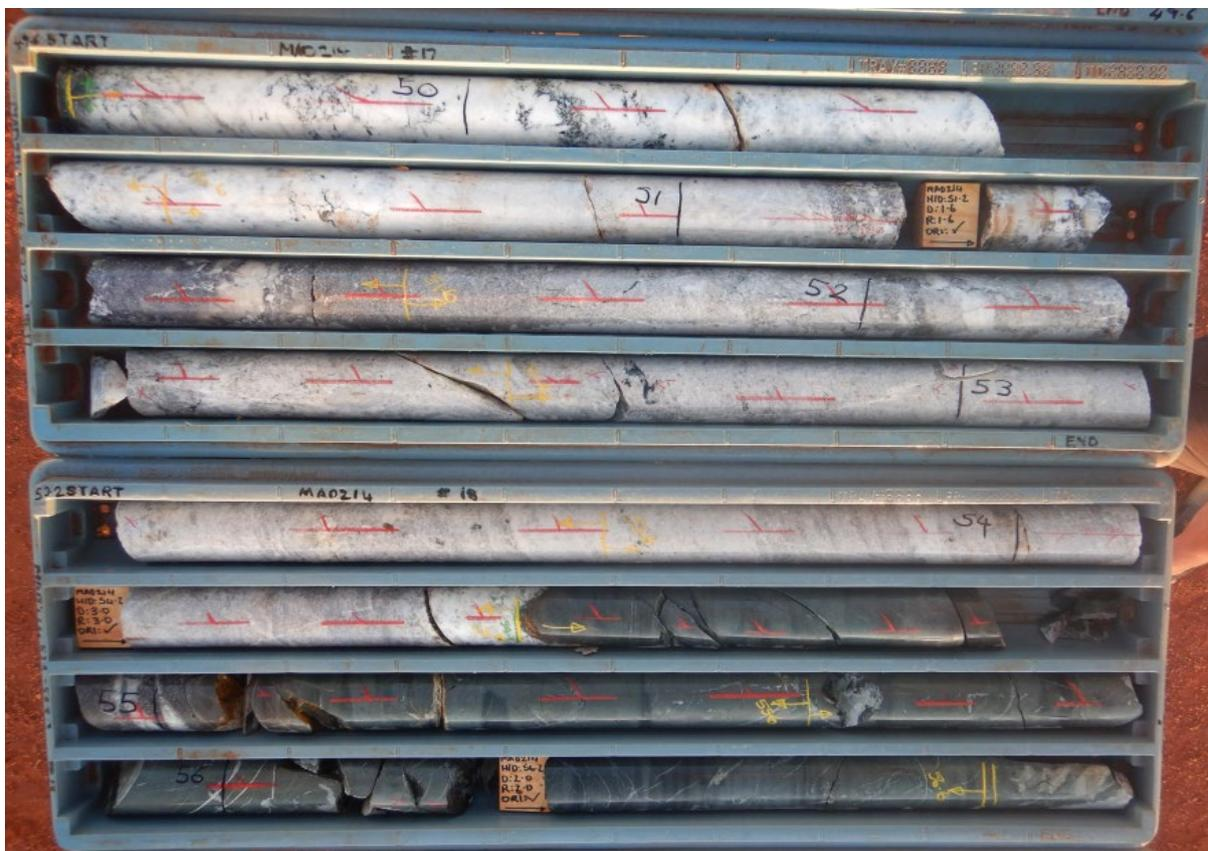
Figure 3 – photo of drill core from MAD214 completed in December 2022 which intersected 5m of pegmatites from 49.5m downhole.
