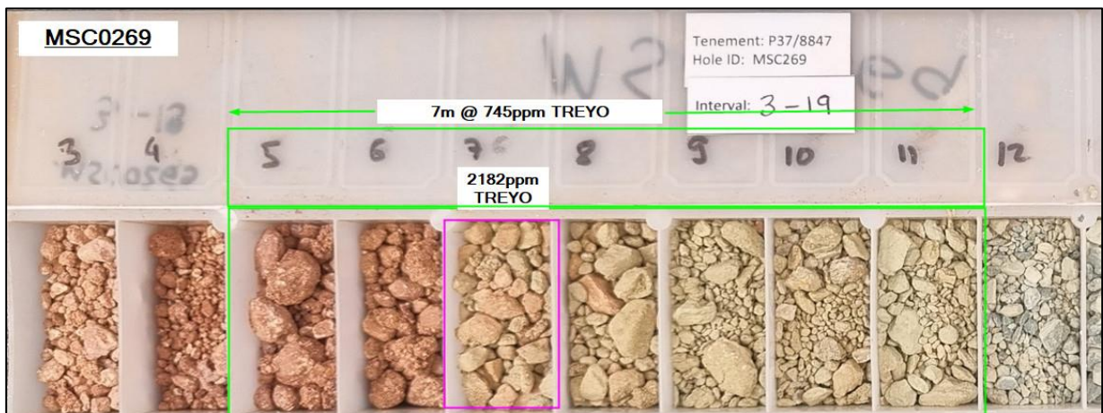
Figure 1 – Yttria Cross Section and RC Chips from high grade TREYO Hole MSC0269
