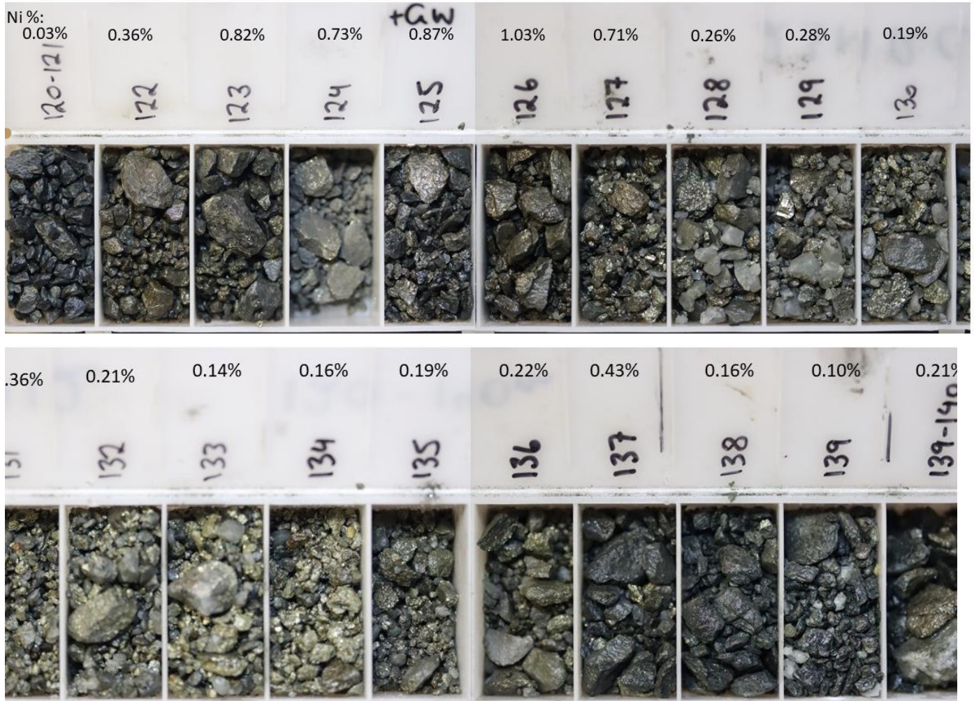
Figure 5: Chips trays from the widest mineralised intersection in 23NRC012, showing nickel grades at each metre.
