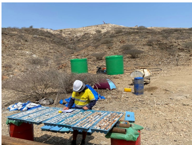
Figure 9: Core-trays laid-out on makeshift core rack at site. Note drill-rig in background on top of hill, set-up on drill-hole NDDH004. Geologist Neil Scholtz logging drill-core from NDDH004.
