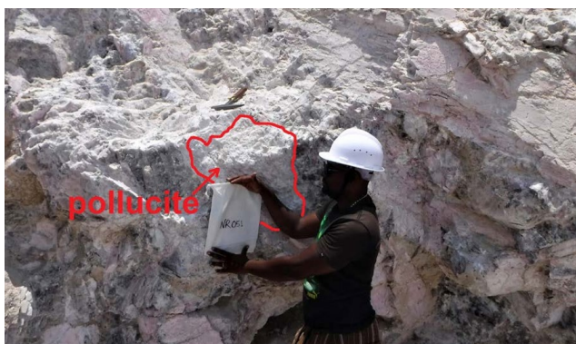
Figure 13: Exposed pollucite mass sampled as NR051. Field and logistics assistant Joao Paulo Boy provides scale
