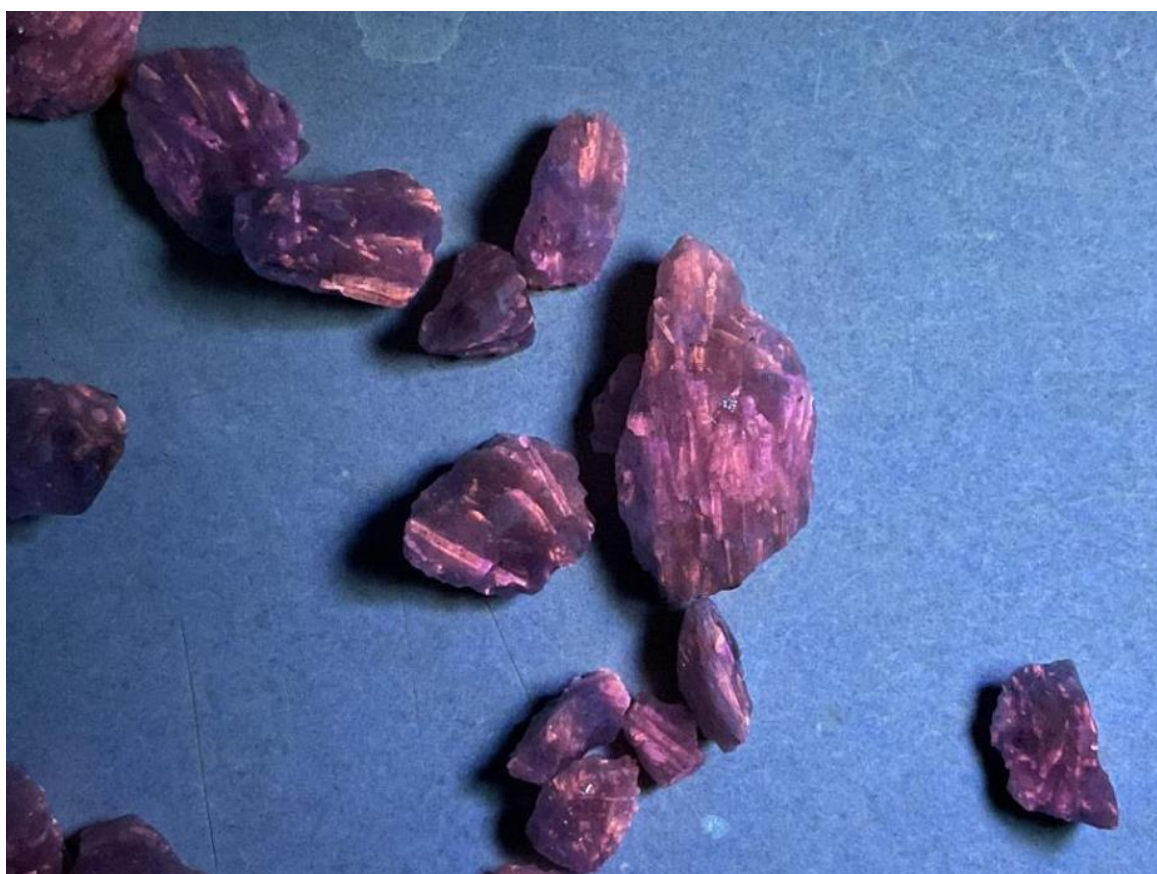
Figure 9: Spodumene crystals in HYRC006 (162-163m) under 250nm ultraviolet light (1m @ 0.47% Li 2 O)
