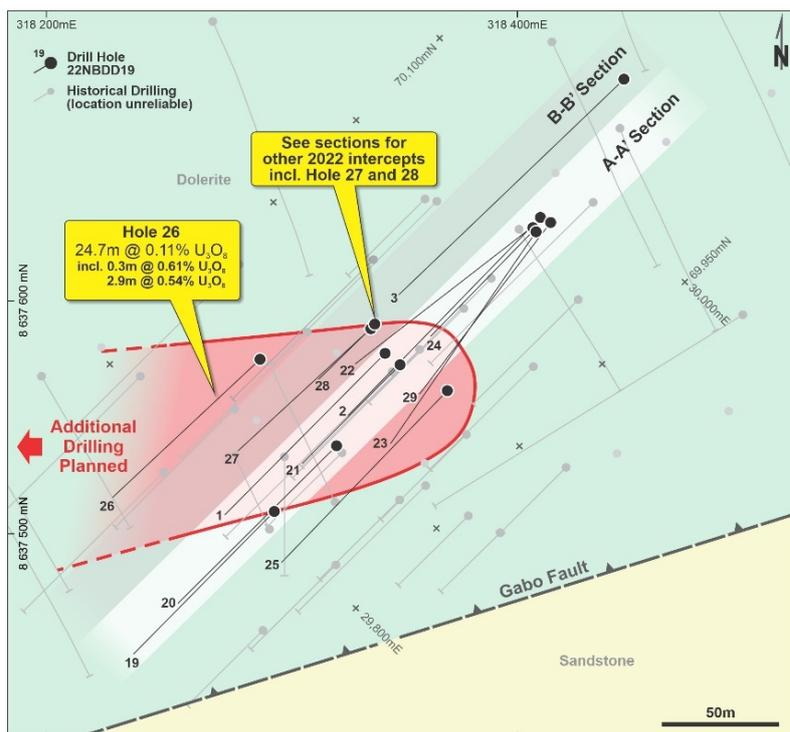
Figure 3: Nabarlek South Prospect – Drill-Hole Collar Plan.
