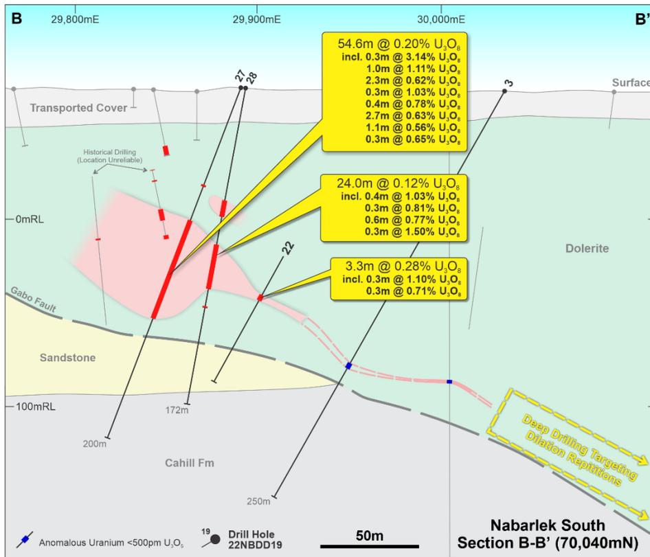
**Figure 1: Nabarlek South Prospect Cross-Section (looking to the north-west).**
