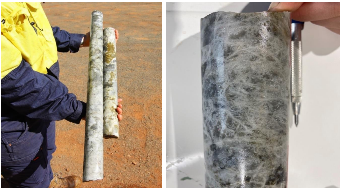
Image 1: Quartz-feldspar-spodumene pegmatite in hole ANDD0201
