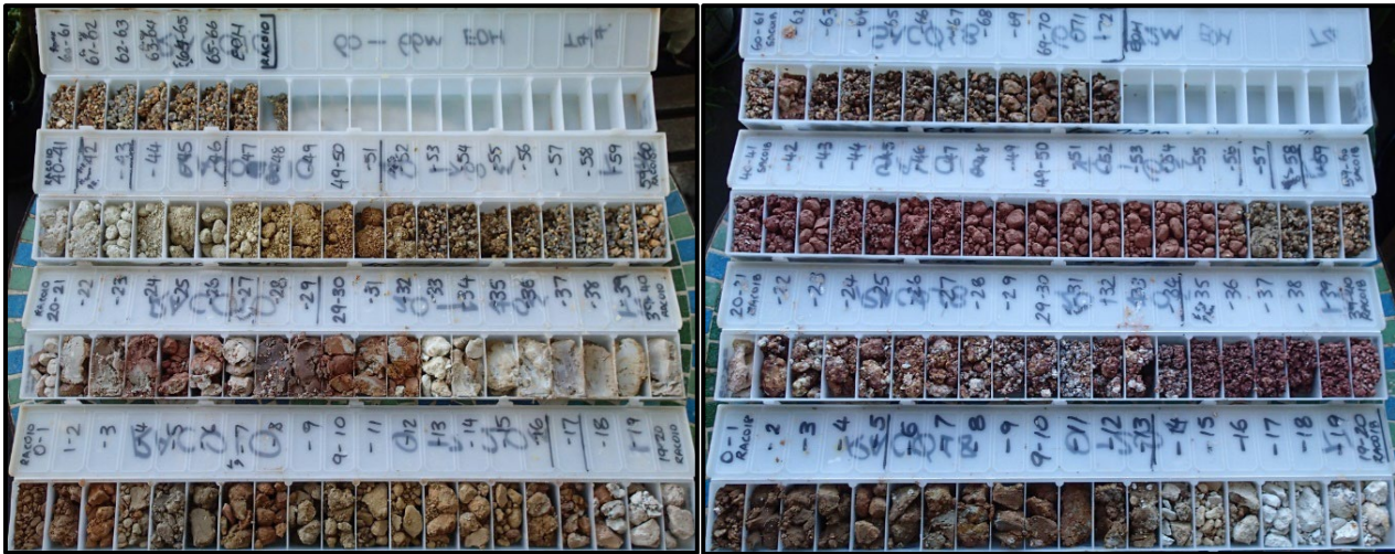
Figure 4: AC chips from RAC010 (66m TD), Ryan Granite (left); and (b) RAC018 (72m TD), Jindera Granite (right) showing red hematitic clays, yellow-orange goethitic material and white clays (pallid zones)
