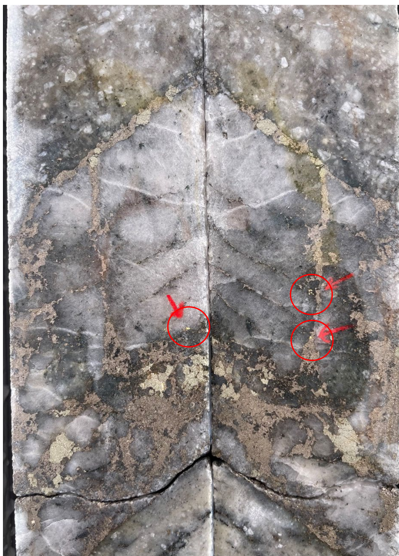
Image 3 – MDRCD660 at 421m down hole, massive pyrrhotite, pyrite and gold
