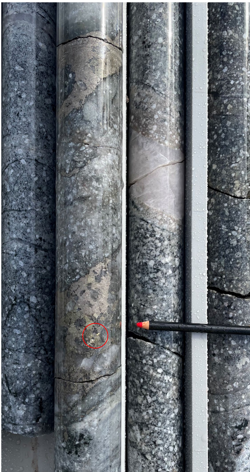
Image 1 – MDRCD660 at 420m down hole, massive pyrrhotite, pyrite and gold
