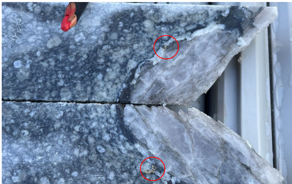
Image 2 – MDRCD660 at 191m down hole, visible gold.
