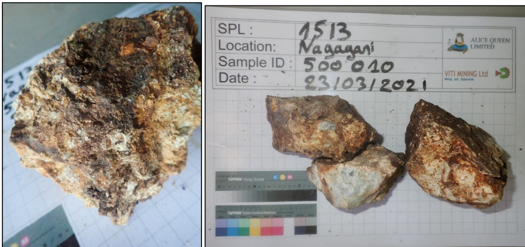
Figure 7. Weathered rock chip samples (alteration and vein) recently collected from the Nagagni and Karikarimasi creek area (Dakuniba Prospect, SPL1513) returning 4.6g/t Au (left) and 1.4 g/t Au (right) collected from an earlier reconnaissance trip.
