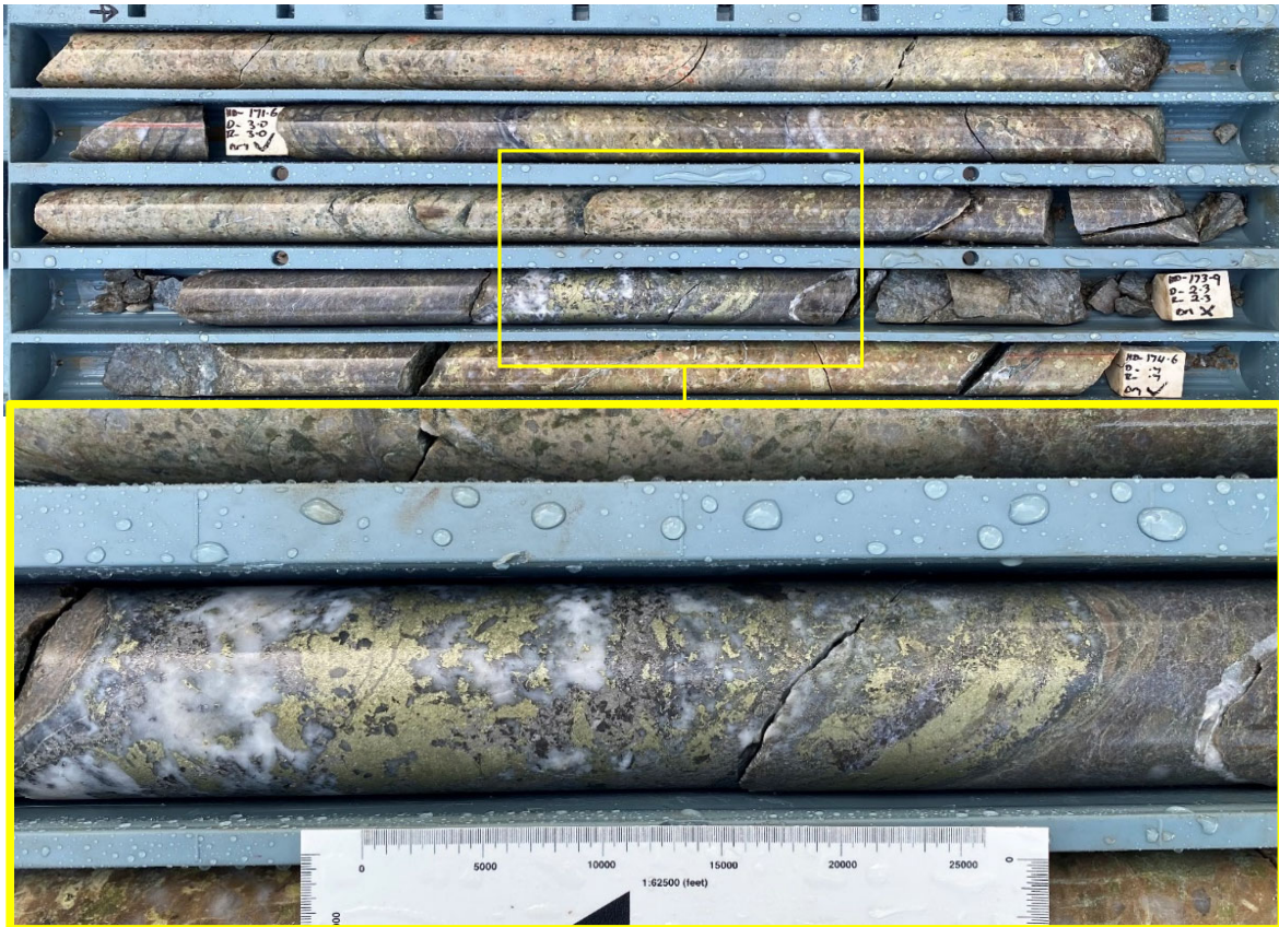
Figure - 14 - From mineralised zone returning 19m @ 0.3 g/t Au from 171m incl. 1m @ 3.5 g/t Au from 181m & incl. 1m @ 3.0% Cu from 173m (22NGD108)
