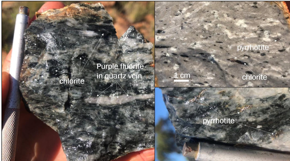
Figure 7: Flow banded felsic volcanic rocks from outcrop (left and lower right 428025E, 6327588N) near the Achilles target showing 50% quartz (white) 49% chlorite (dark green) banding with 1% volatile mineral fluorite (purple) in a quartz vein. Top right photo (427562E, 6329036N) displaying squashed vesicles (air bubbles) filled with the iron sulphide mineral pyrrhotite 2% and alteration mineral chlorite 8% in grey quartz feldspar aphanitic groundmass. These uneconomic elements in fluorite and pyrrhotite are considered important in transporting mineralisation in hydrous magmas as they contain volatile elements and hence demonstrate the fertile nature of these volcanic magmas refer Blevin, 2004
