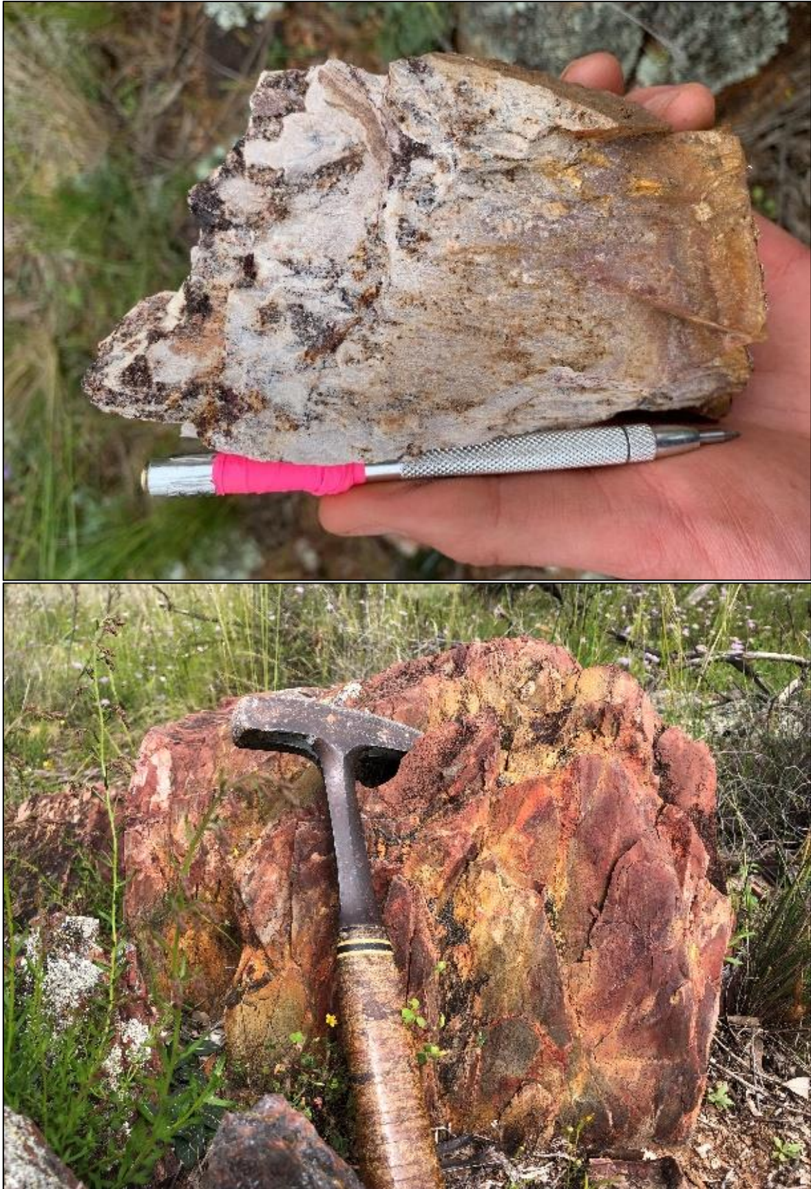
Figure 9: Photographs of outcrop (top 429877E, 6346640N; lower 429874E, 6346629N) with strongly sericite-chlorite altered marine siltstones (Dssa) within volcanosedimentary rocks along the Planet trend. Both exhibit boxworks after pyrite 5% has oxidised out. Pyrite is not a mineral of economic interest, rather in this setting it is a mineral indicating the presence of hydrothermal activity.
