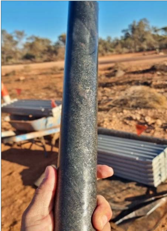
Photo 2: Heavy disseminated sulphide intrusion from RKDD081 from 840m, NQ2
