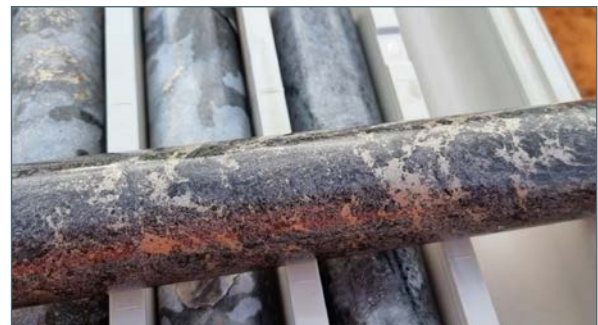
Photo 5: Heavy disseminated and net-textured sulphide from RKDD083 from 751m, NQ2
