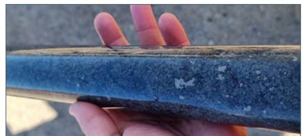
Photo 8: Ni-Cu sulphide mineralisation from RKDD085 from 237m downhole
