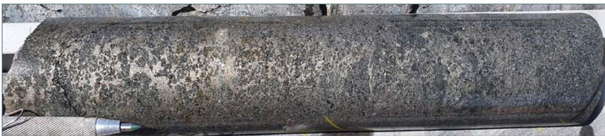
Photo 1: Net-textured and heavy disseminated Ni-Cu sulphide from RKDD033 from 394m, NQ2
