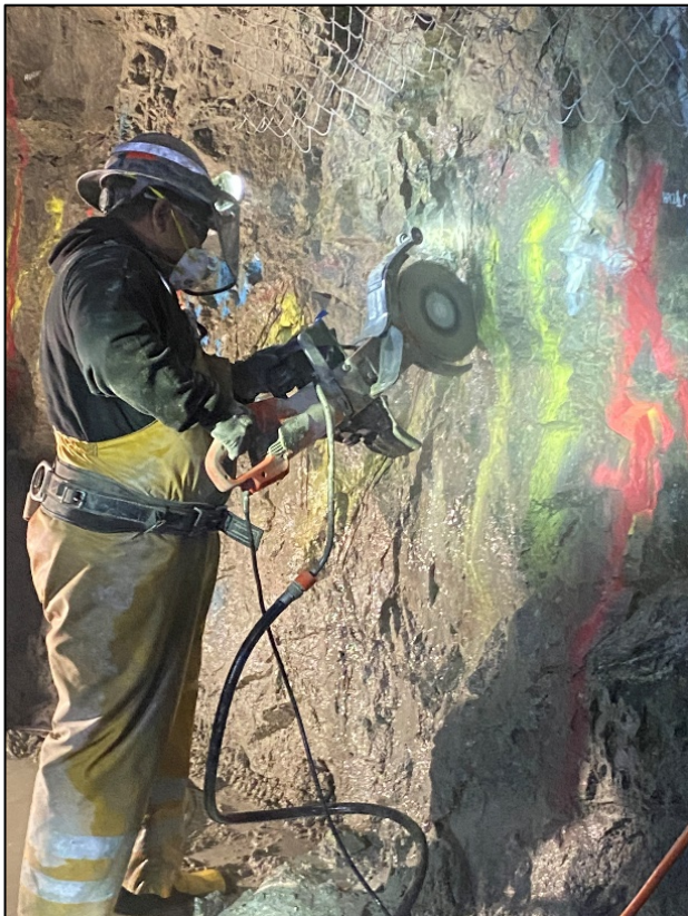
Photos 1 and 2 – Channel sampling of underground walls showing exposed mineralisation. Note sample width is approximately 2.5cm.
