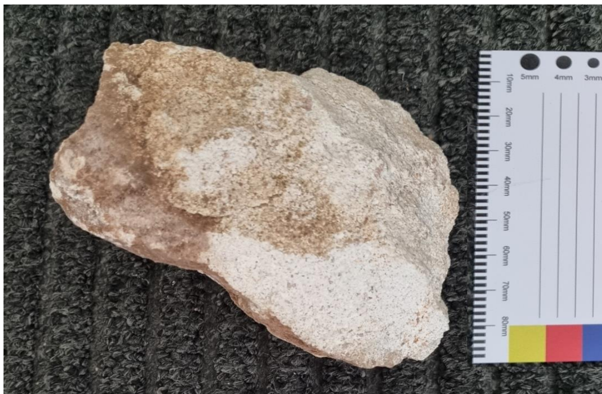
Figure 2 Sample VK-094 with 36.6% halloysite content
