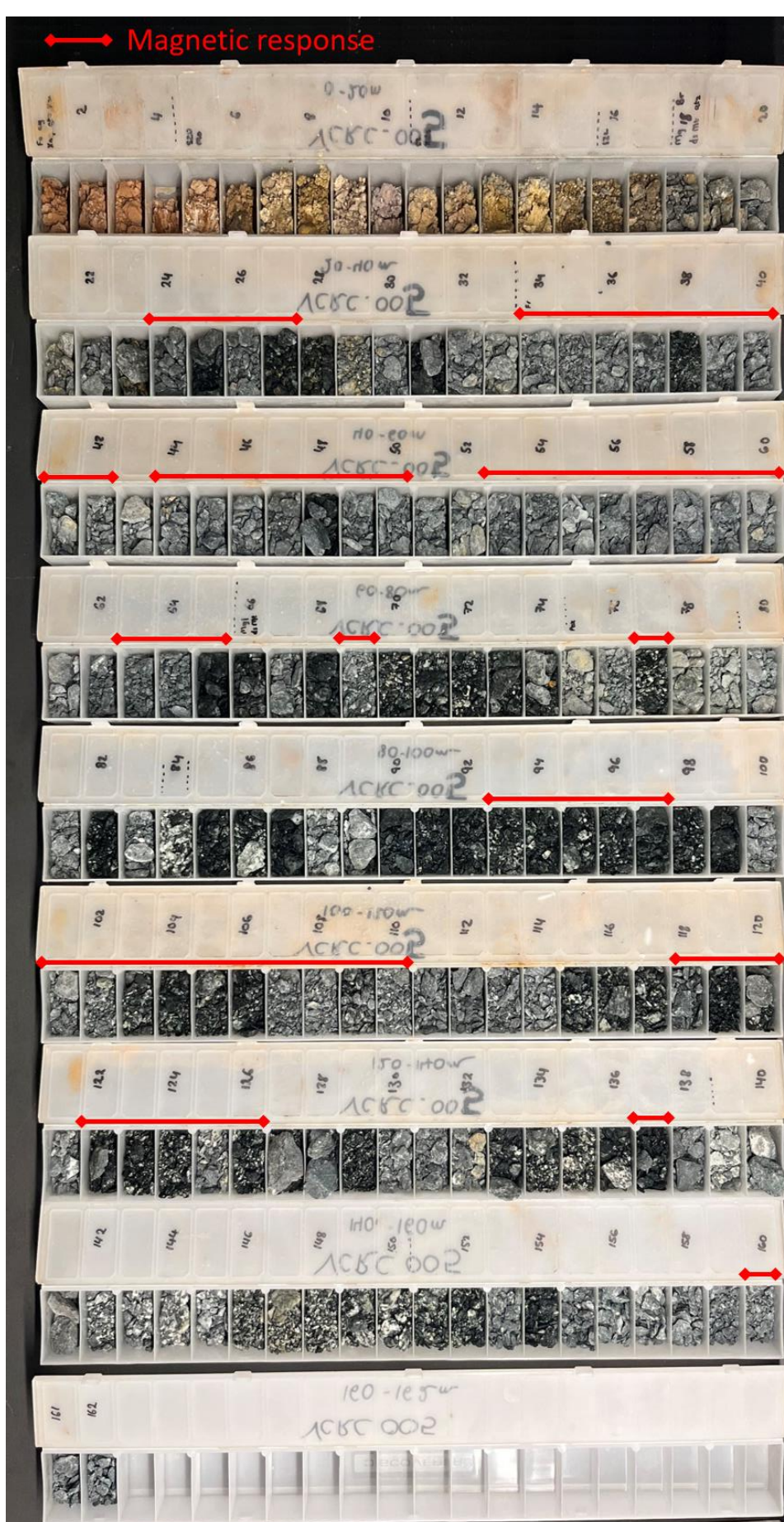
Figure 6; RC chips from hole VCRC0005 with horizons which have a magnetic response annotated. Depths downhole are written on the chip trays with each compartment representing 1m downhole interval, commencing from top of hole to 162m depth. Each tray contains 20m of chips.
