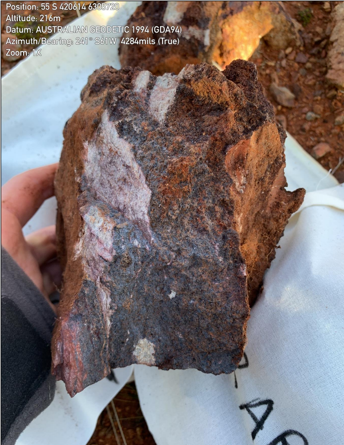
Figure 8: Gossanous rockchip sample RARC004 from the outcrop in figure 7, RARK004 graded 3.5g/t gold, 33g/t silver, 1% lead + zinc, 800ppm copper, 24ppm molybdenum, 60ppm bismuth, 1585 arsenic, 18ppm indium.
