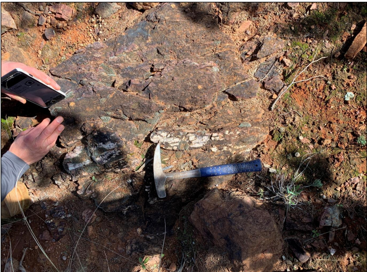
Figure 7 Rockchip sample location RARCO04 prior to sampling showing gossanous brown rock and white quartz veins, hosted in foliated ex-sulphide bearing sediments and near the eastern contact with coherent rhyolite (out of picture).
