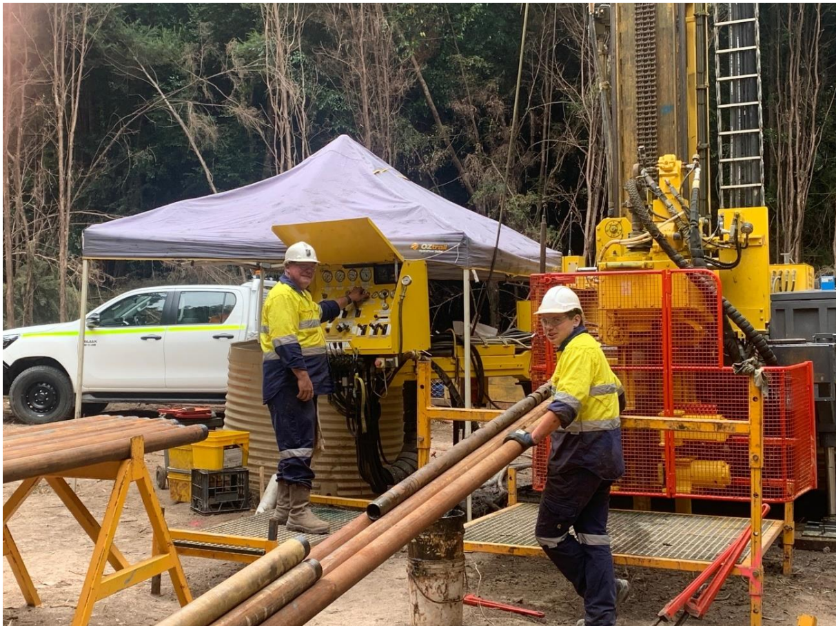
Figure 1: Diamond Drilling at Arthur River prospect
