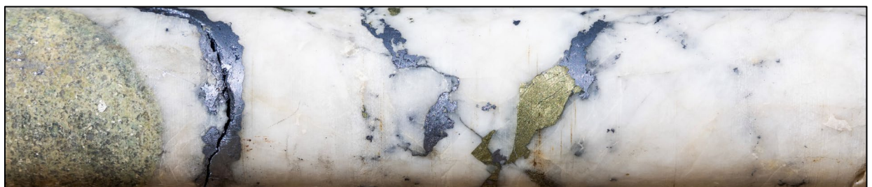
Figure 1: Quartz vein with abundant molybdenite, chalcopyrite and pyrite from 21TVDD001 (338.1m).
