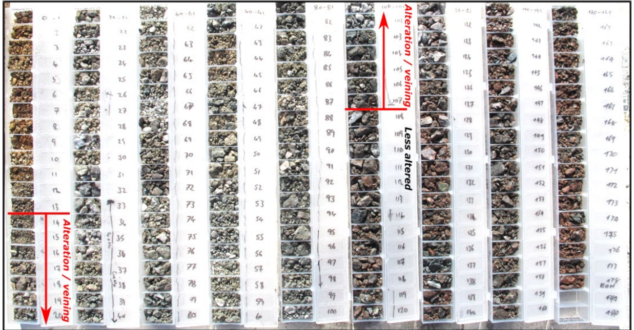
Figure 4: Quartz veining and sericite alteration (light colour) in 21TVRC001 RC chips.
