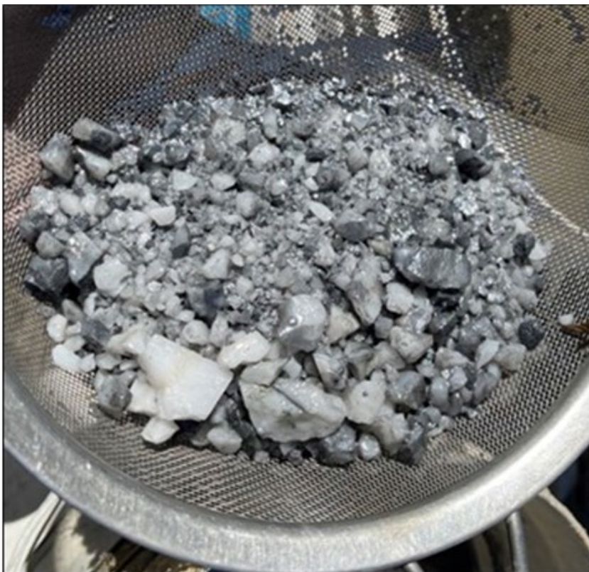
Figure 3: Sieve of quartz and molybdenite from RC drilling at Titov (21TVRC004, 74-75m).
