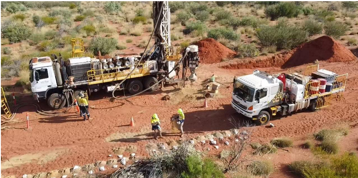
Figure 1: RC drill rig in operation at the West Arunta Project
