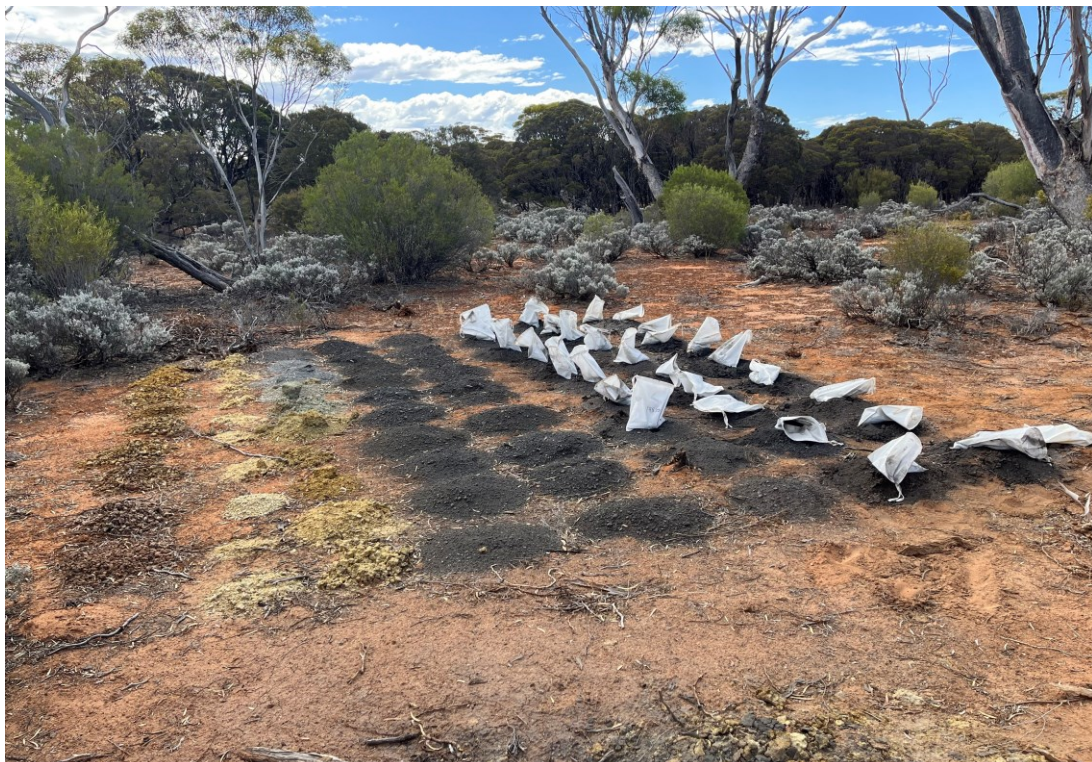
Figure 2. Re-split samples collected from the sample piles for air core hole 22DAC073.
