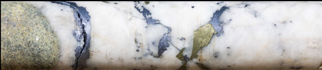
Quartz vein with abundant molybdenite, chalcopyrite and pyrite from 21TVDD001
