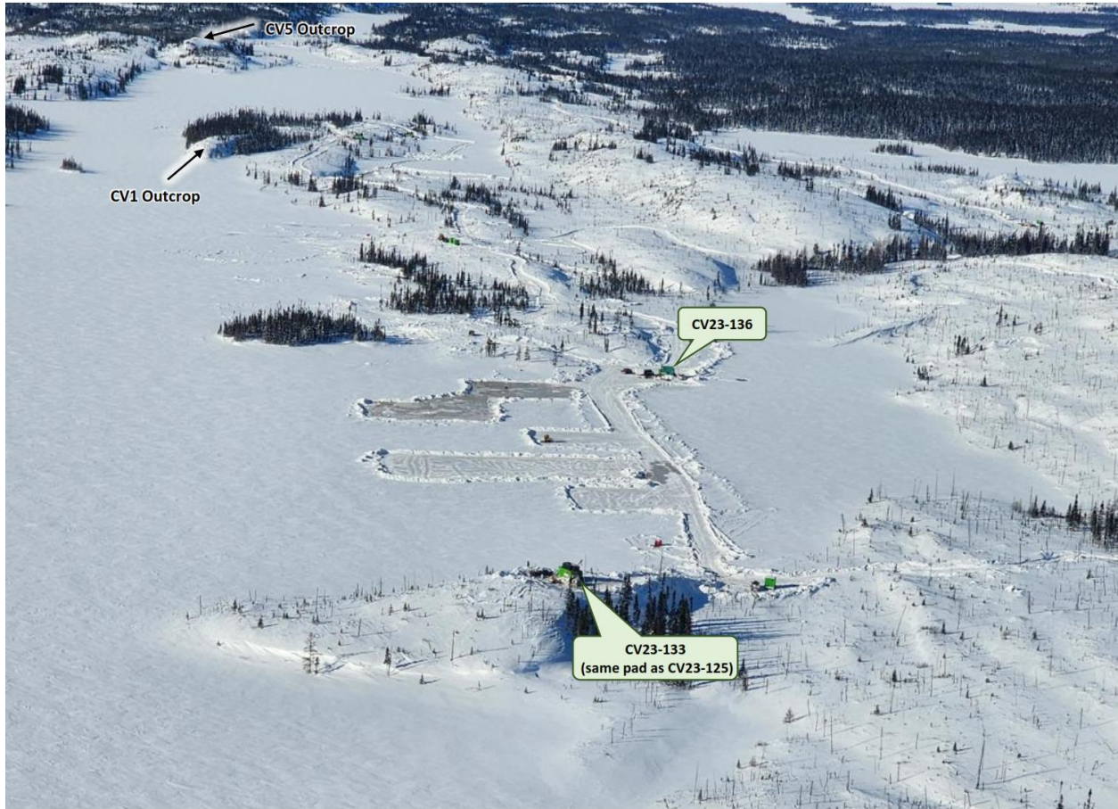
Figure 3: Lake-ice pad preparation for drilling completed over newly defined 550 m strike length at CV5
