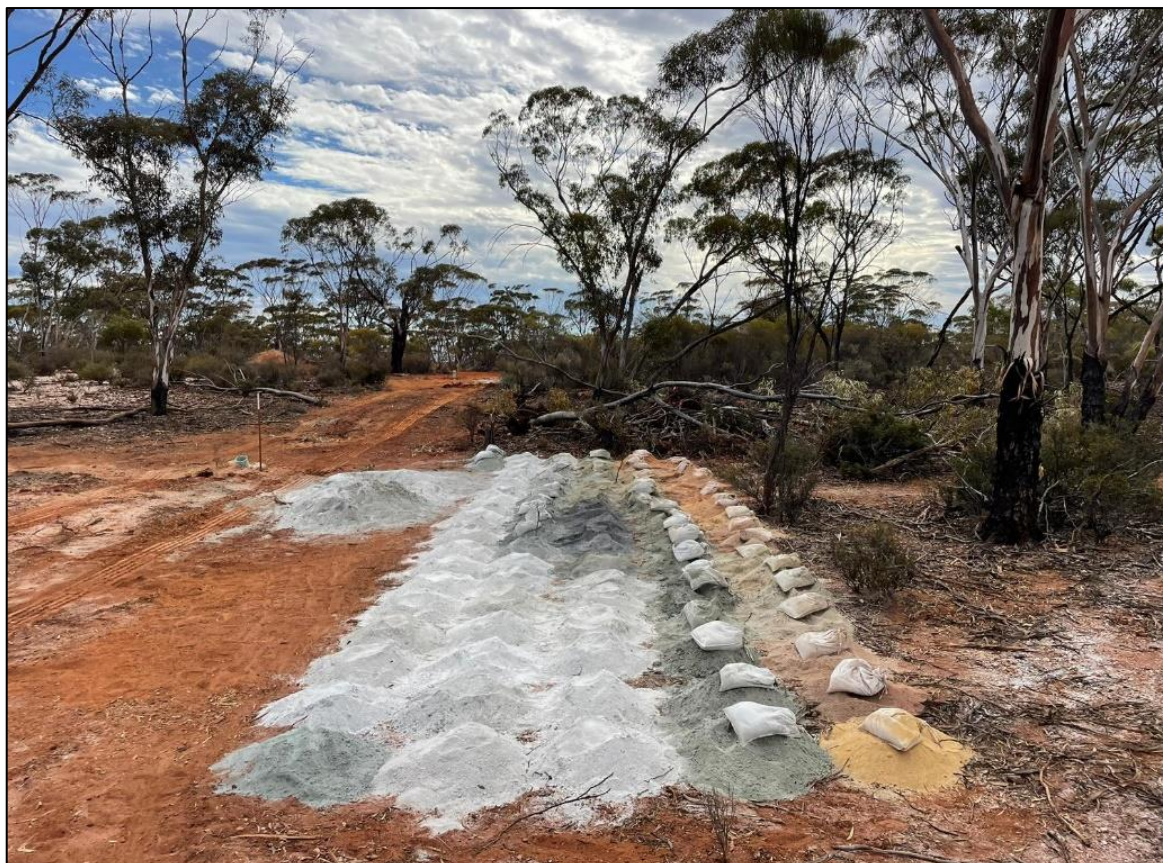
Figure 3 - Drill spoils from hole 23RC031 showing wide zone of pegmatite (white samples)
