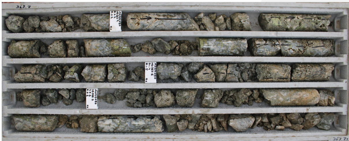
Figure 3. MHDD080 Drill Core Showing Vuggy Transition Zone Chalcopyrite-Pyrite and Chalcocite Mineralisation.
