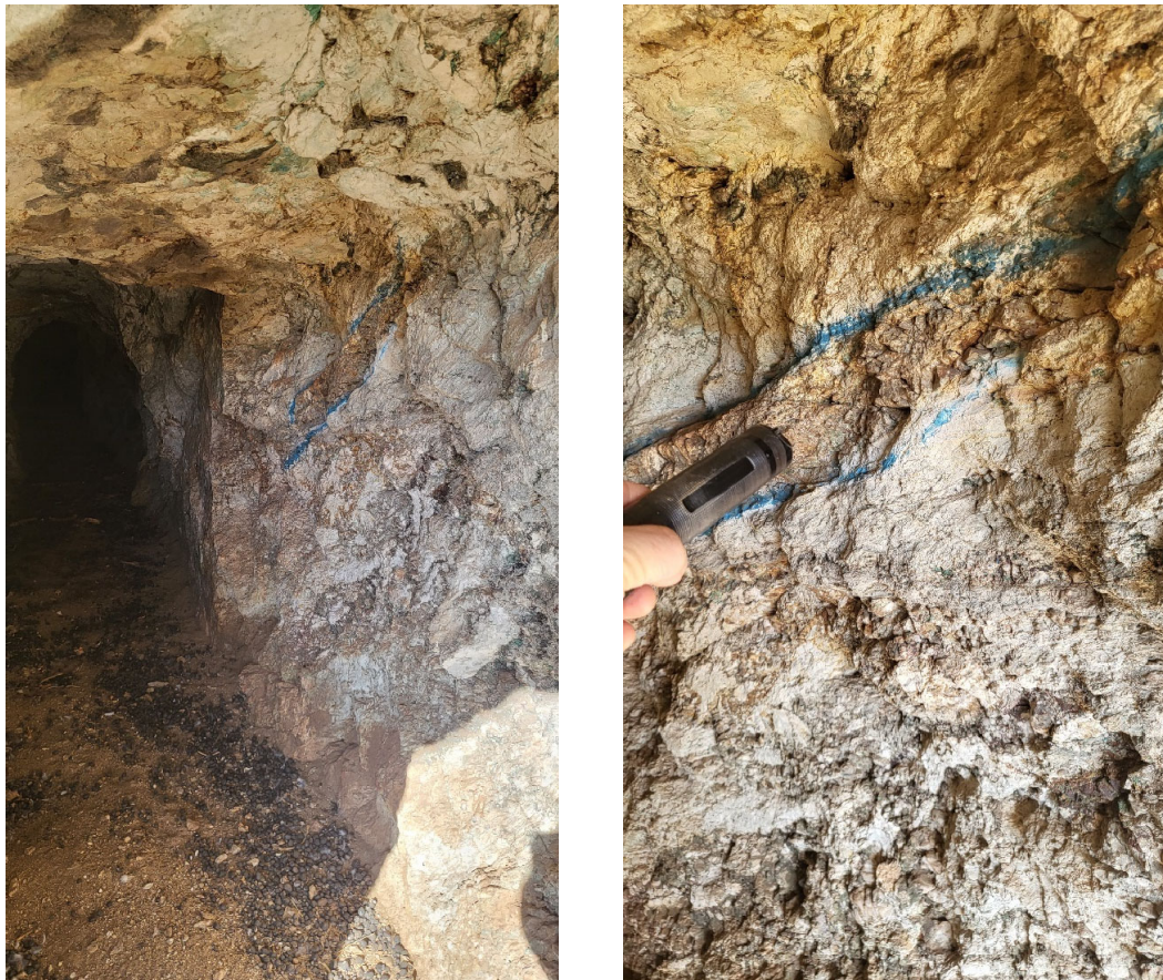
Figure 7: Field photograph of the historical adit at Tombstone (left) showing two bedding-parallel azurite veins (blue mineral) and a close-up (right) of the same two veins.
