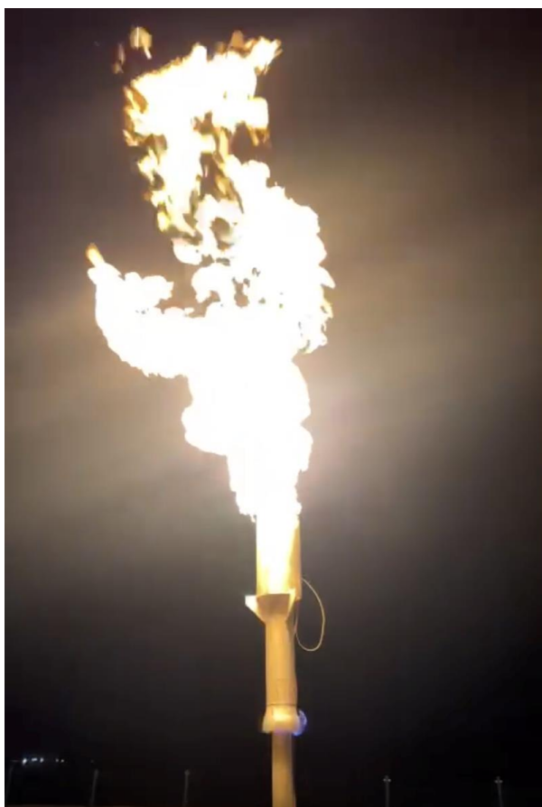
Figure 1 – Red Lake-5 gas flare generated from the annulus of the well
