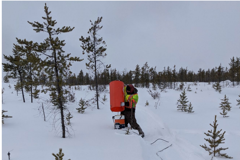
Figure 2 –Step-Wise Moving-Loop Transient Electromagnetics Survey SQUID Sensor
