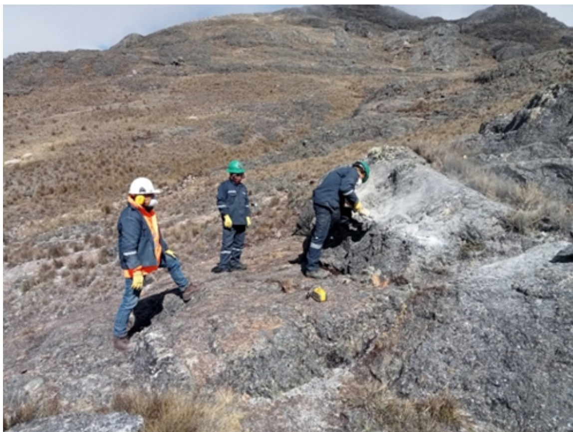
Figure 6. Surface sampling of a mineralised structure, cutting a continuous channel with a diamond blade.
