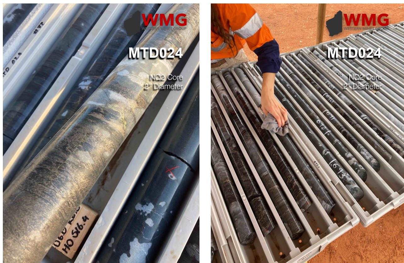
Figure 1: Photos showing examples of sulphidic black shales in hole MTD024
