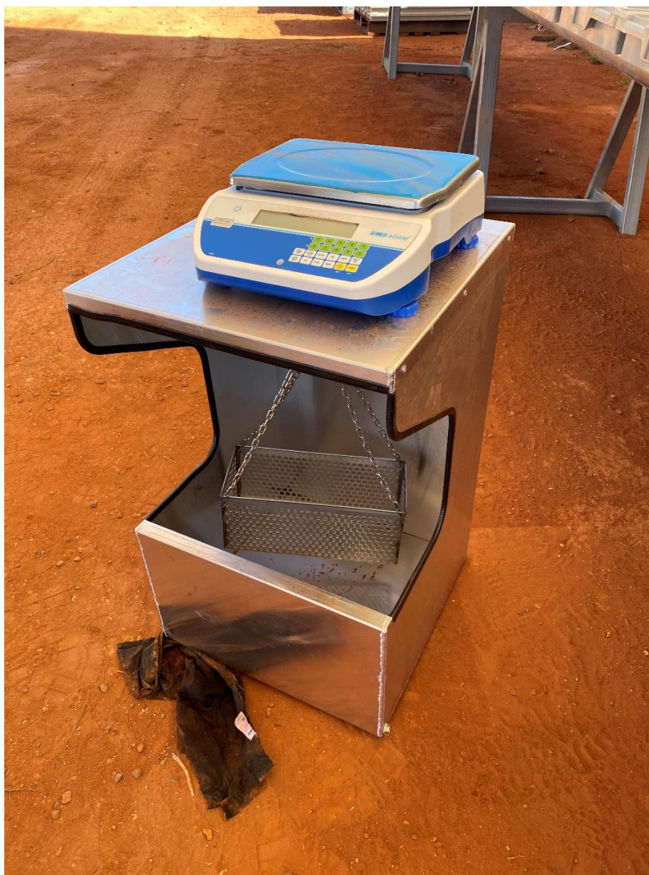
Figure 9-2: Density Measurement setup on site.
