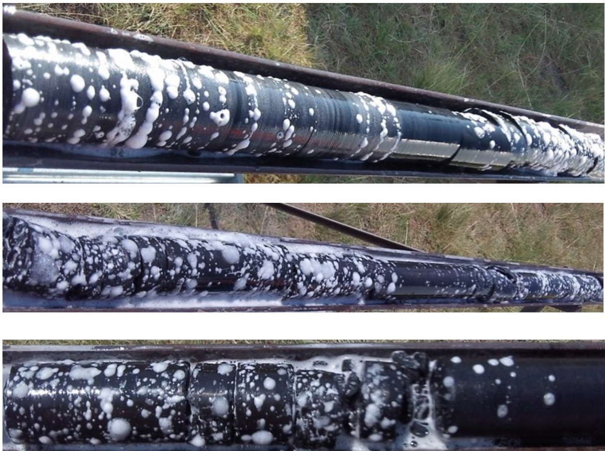
Figure 1: Core well 270-05C visible gas emissions observed from representative core samples at depths between 175-287m
