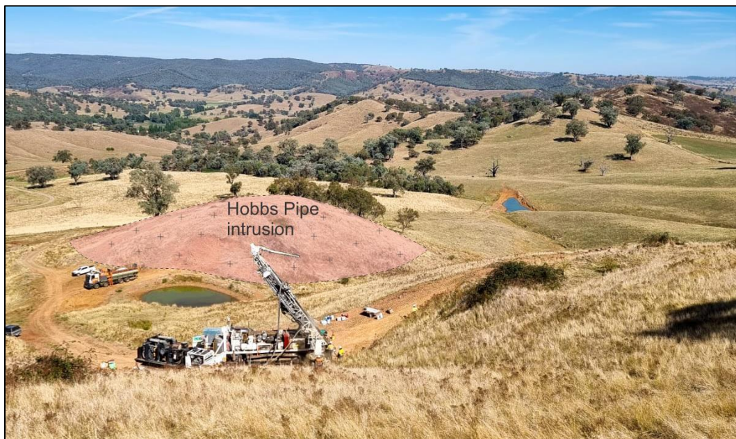
Figure 1 – Durock Drilling's track-mounted RC rig has commenced drilling at Greater Hobbs Pipe area to complete Phase 2 of the drill program at the Mt Adrah Project, Lachlan Fold, NSW.
