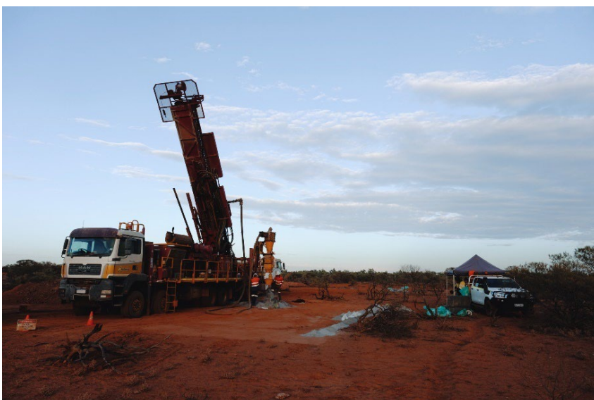
Figure 1: Photo of the RC rig drilling undercover ironstones to the south of the Yin Resource.
