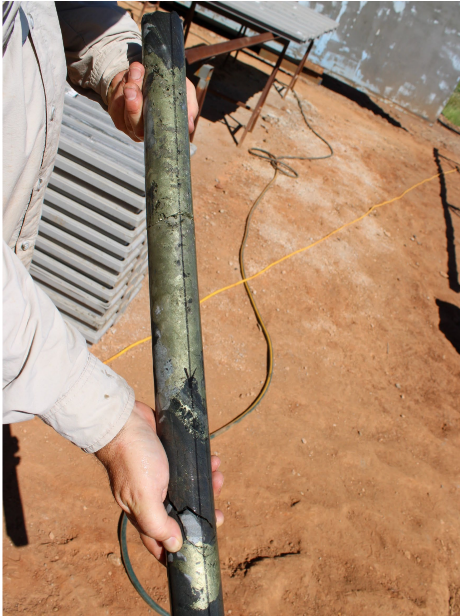
Figure 5. Massive chalcopyrite copper mineralisation in MHDD010 from 269.1m to 269.65m
