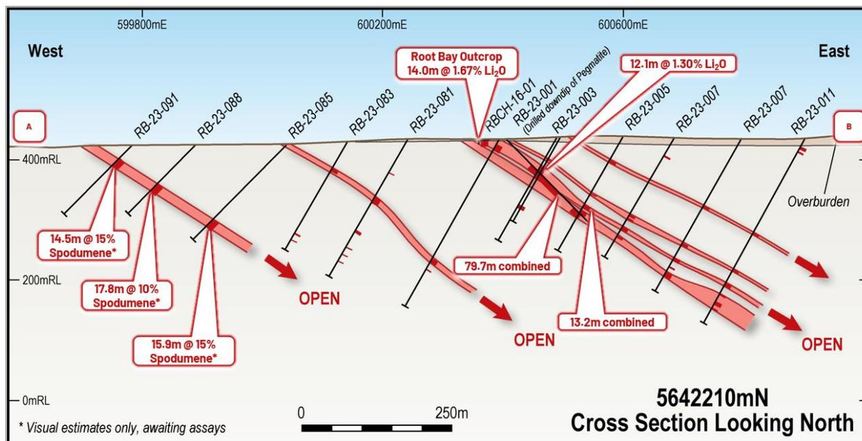
Figure 1. Cross section A-B along first fence line drilling
