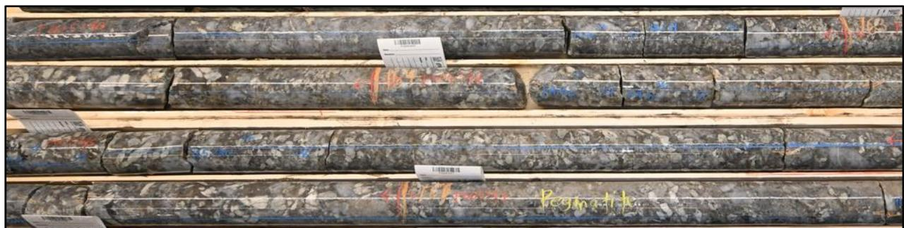
**Figure 3.** RB-23-001 - NQ diamond core showing high density spodumene crystal laths, 7.3m @ 1.44%  $\text{Li}_2\text{O}$  from 162.0m
