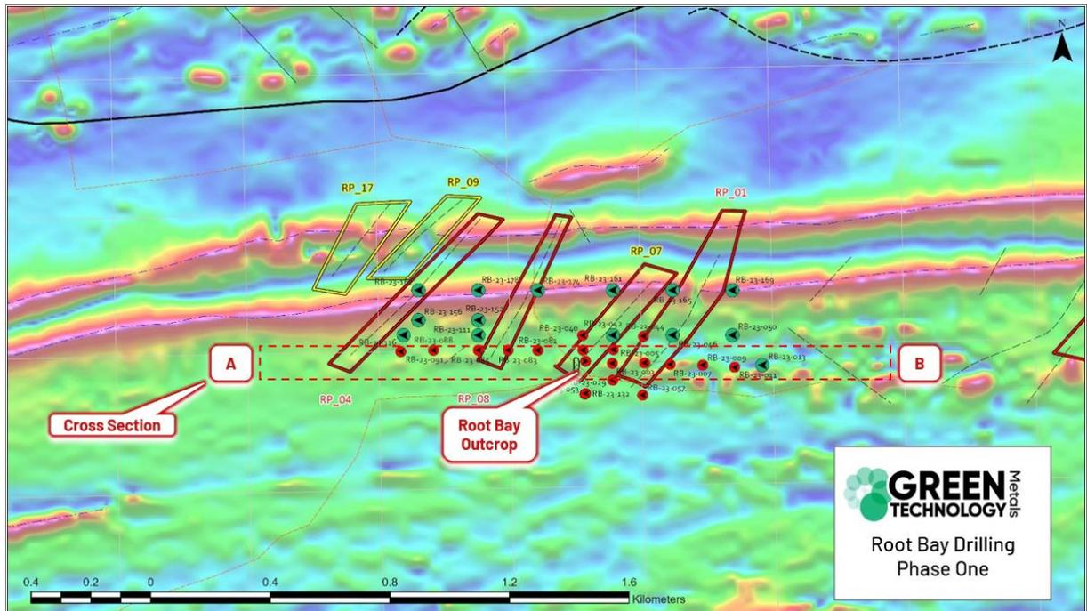
**Figure 2.** Litho-Structural Interpretation and Drill collar location (red = drilled, green = planned) base map magnetics, polygons geophysical targets
