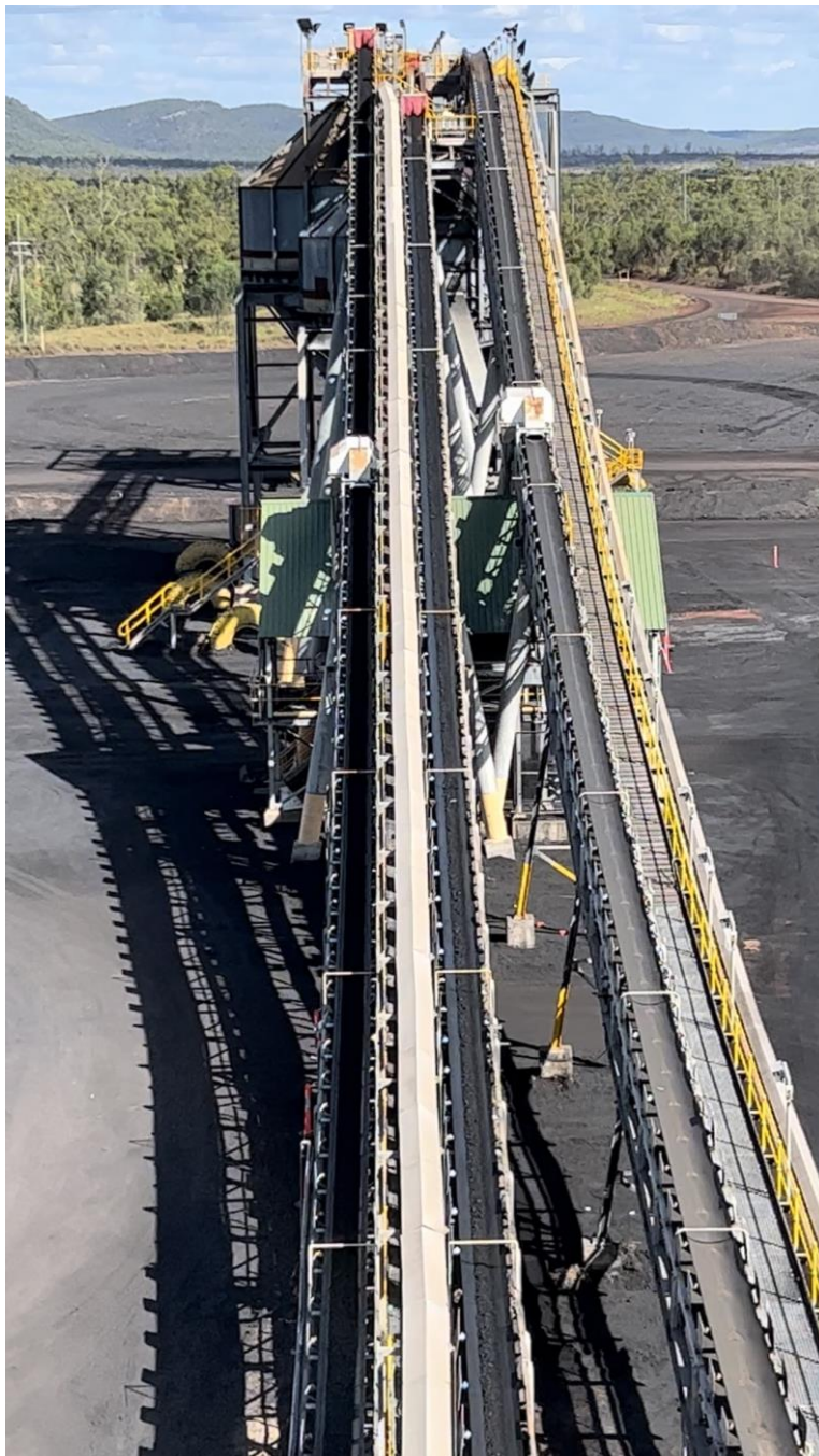
Figure 2. Product coal from Module 1 of the refurbished Burton CHPP. (Left two conveyor belts)
