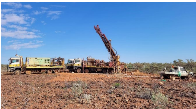
Figure 1: Photo of the RC rig drilling at C3.
