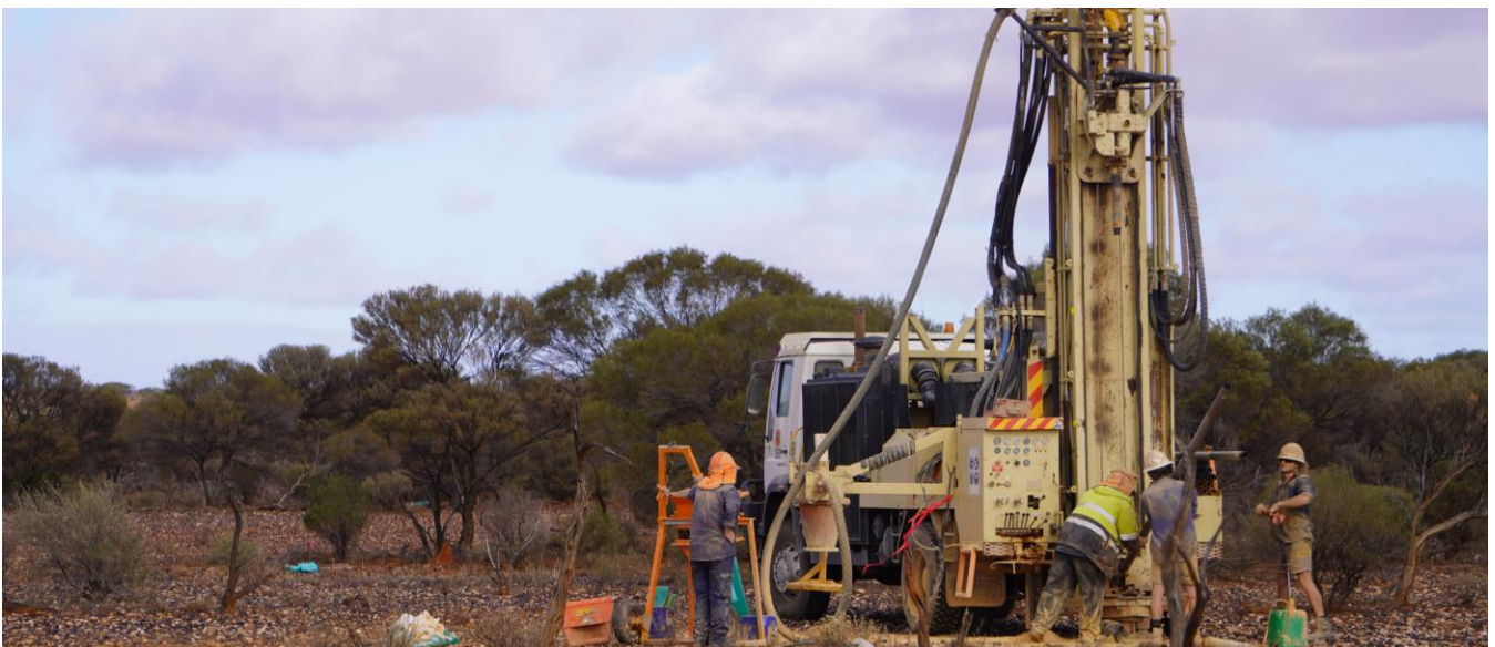
Figure 6: Reverse circulation drilling at the Company’s Flagship Mt Stirling Project.
