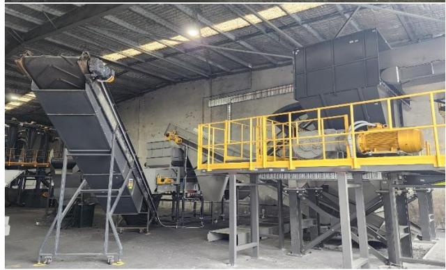
*IMAGES 5 to 7: Inline shredder installation at Stapylton: Source Company*
